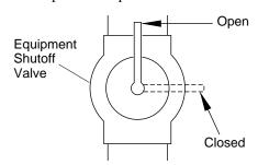
Figure 13 - Equipment Shutoff Valve
